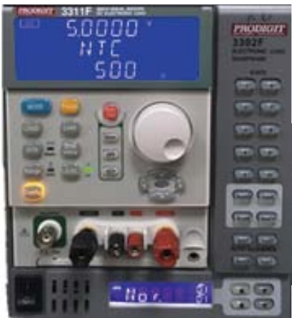
3302F frame with NTC module set NTC resistance is 500K \Omega
