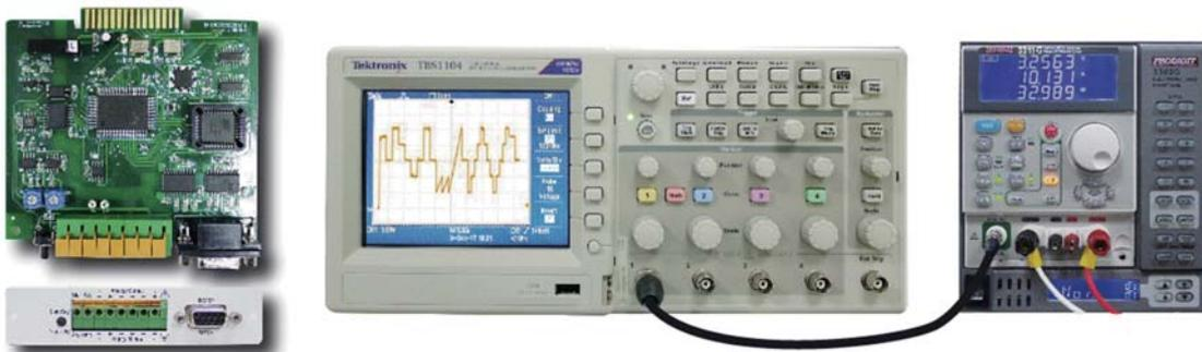
The new Model 9923 Current Waveform Generator (Option) provides real battery discharge current waveform simulation. This option installs in Model 9923 to 3302G, 3305G and 3300G Series load mainframes and can simulate real battery discharge current waveforms.
