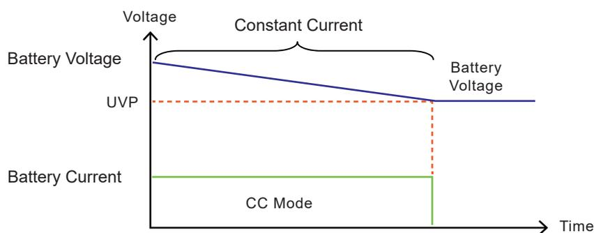
Figure 6 : CC + UVP mode battery discharge test
