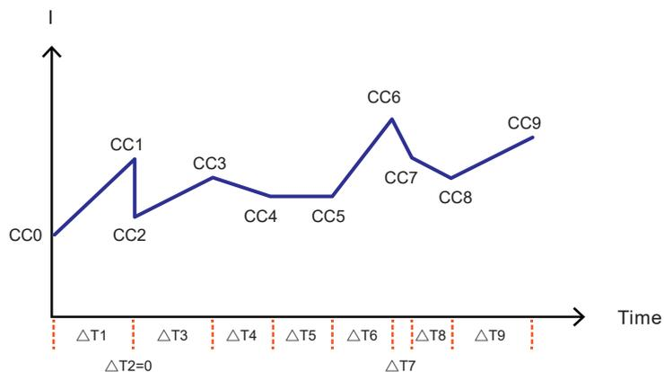
Figure 10 : Ramp mode battery discharge test
