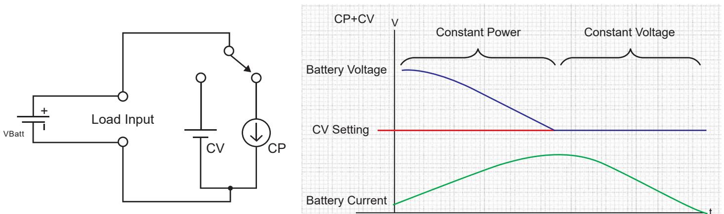
Figure 5 : Application of CP+CV operation mode
